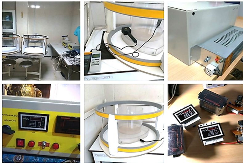
Figure 1: Different parts of electromagnetic generators
