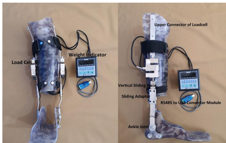
Figure 2: Patellar tendon-bearing (PTB) brace with indicator of off-loading amount on tibia
