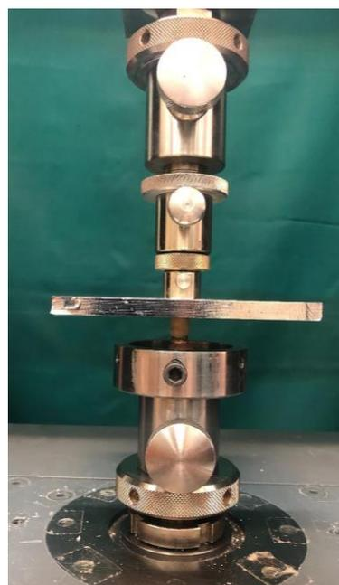
**Figure 5:** The crowns clamped in the holder of a universal testing machine and loaded vertically on the occlusal surface
