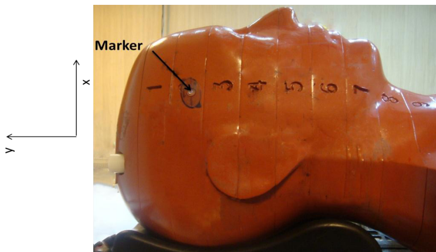
Figure 2: RANDO phantom and the position of the marker used in skin dosimetry of parotid cancer
