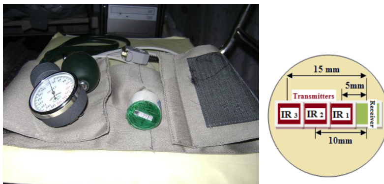
Figure 1: Optical transmitters and receiver position in the optical system
