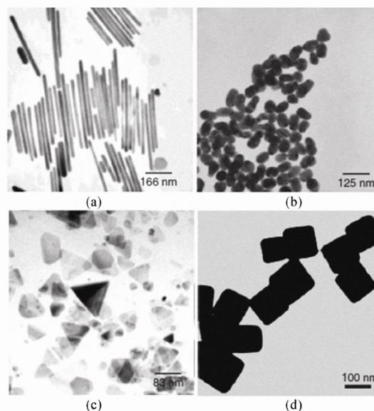
**Figure 3:** Nanoparticle geometries: a) Gold nanorods, b) Gold colloids, (c) Silver triangular prisms, and d) Silver nanocubes [47].
