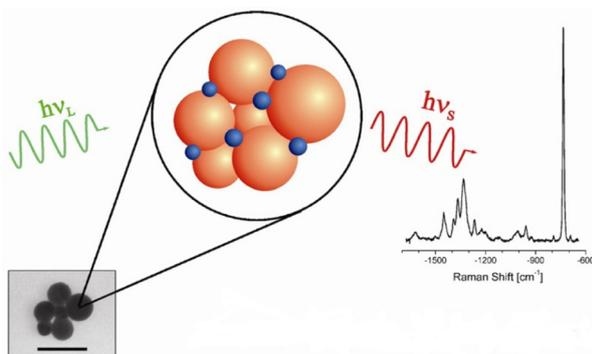
**Figure 2:** Schematic diagram of SERS [4].
