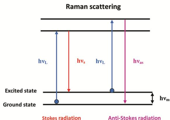
**Figure 1:** Schematic diagram showing Raman scattering.
