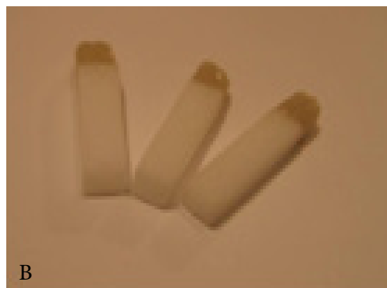
Figure 1: A. zirconia-based blocks (Zirkonzahn, Steger, Ahrntal, Italy) prepared at 4x4x12 mm dimensions. B. Three brands of veneering ceramics used for layering the zirconia cores.
