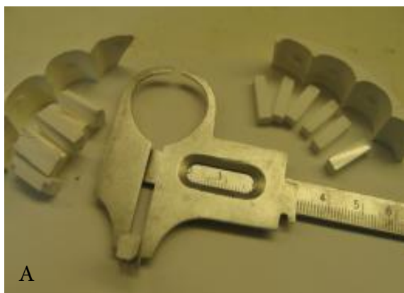
Figure 1: A. zirconia-based blocks (Zirkonzahn, Steger, Ahrntal, Italy) prepared at 4x4x12 mm dimensions. B. Three brands of veneering ceramics used for layering the zirconia cores.
