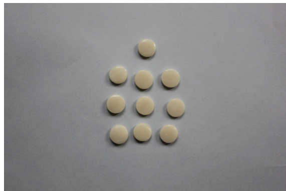
Figure 1: Disc shape specimens with 10 mm in diameter and 2 mm in thickness.
