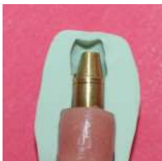
Figure 2: The putty index to ensure that the dimensions of all specimens are identical
